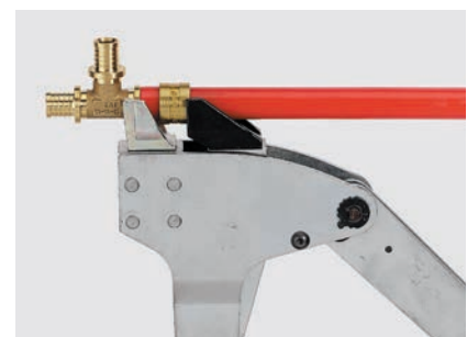
Manual push-on connection process with KSZ.
